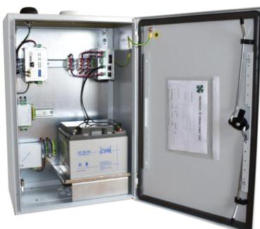
Completed OFF-GRID system has met and exceeded the goals we set out before development began. The system is able to protect the remote object, while running the control program and securely providing the data to the remote users. The extreme summer heat and a series of storms also showed its high resistance to extreme weather.
